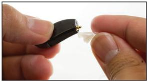
• Disconnect the sound tube by pulling it firmly away from the device. (Do not pull on the thin tube)
